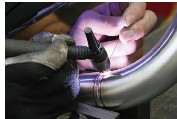
TIG Welding stainless steel elbow.
