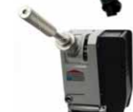
Adjustable grinding angel from 15-180°
